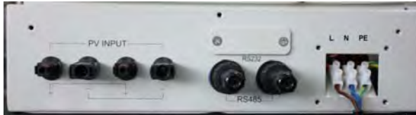
Fig. 7 Connections available on inverter bottom and relevant marking
